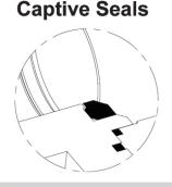
Detail of Protected seat & encapsulated body seal design. Isolates & protects both seats and seals from flow path. Helps to prevent cold flow.
